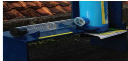
Figure 3. Results of the development of a liquid density measuring instrument integrating fluid pressure and spring elasticity
